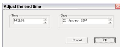
Click the **Adjust** button next to the start or end time and enter the precise start (or end) time and date in the dialog box that appears.
