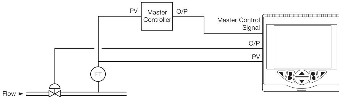
Fig. 23: Auto / Manual station and analog backup station
