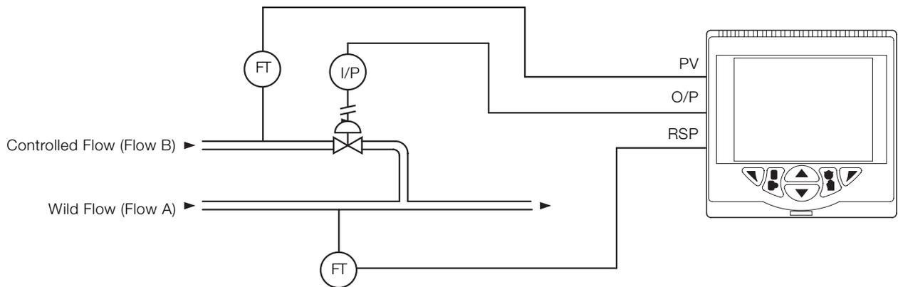
Fig. 21: Ratio controller
