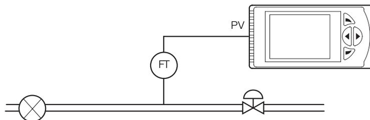
Fig. 12: Single PV with totalization
