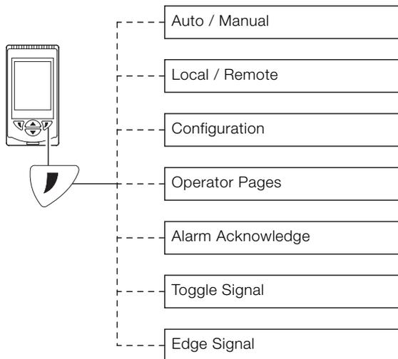
Fig. 5: Programmable soft key
