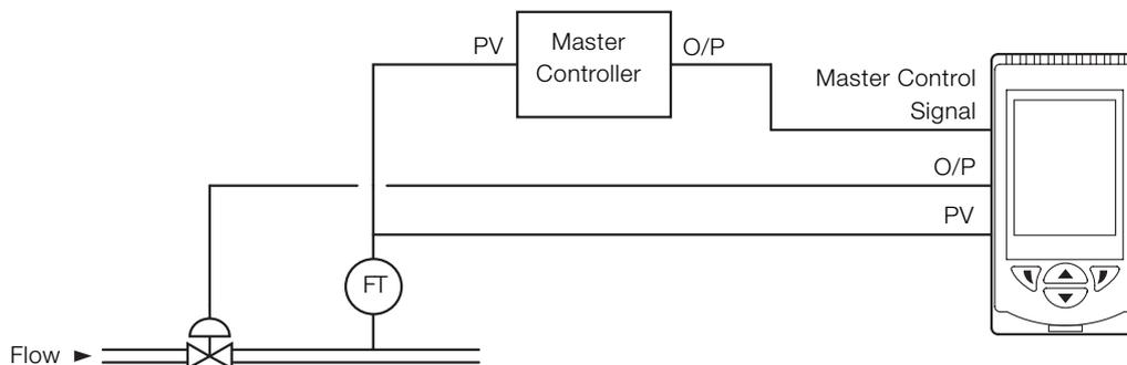
Fig. 15: Auto / Manual station and analog backup station
