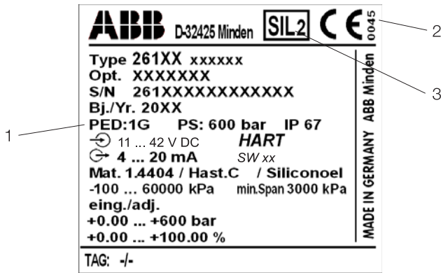
Fig. 3: Identification codes according to Pressure Equipment Directive (example)
